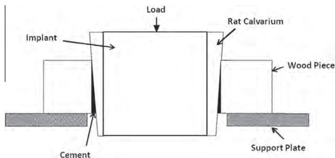
Fig. 2. Schematic of the method used to determine push-out strengths.
