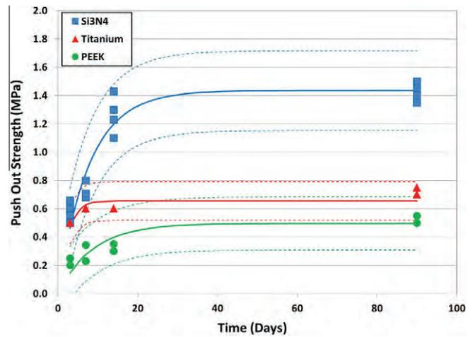
**Fig. 3.** Implant push-out strengths without bacterial inoculation: Nonlinear regression analysis using the simplified Boltzmann equation. Dashed lines represent 95% confidence interval.
